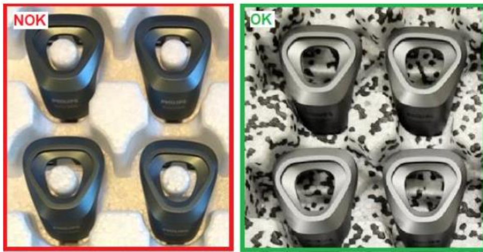
Figure 45. Example of a tray that does not allow gripping from the inside of the workpiece (left)
