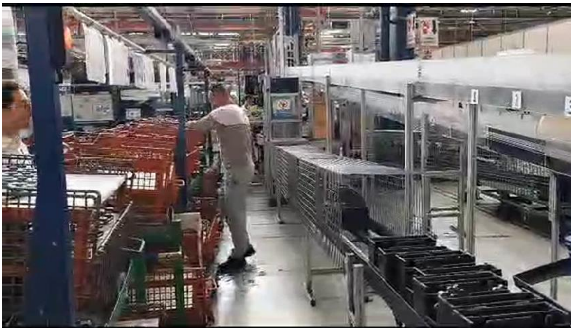
Figure 25. Operator taking a component from the input container (left side). It will then put on the destination container (right side)
