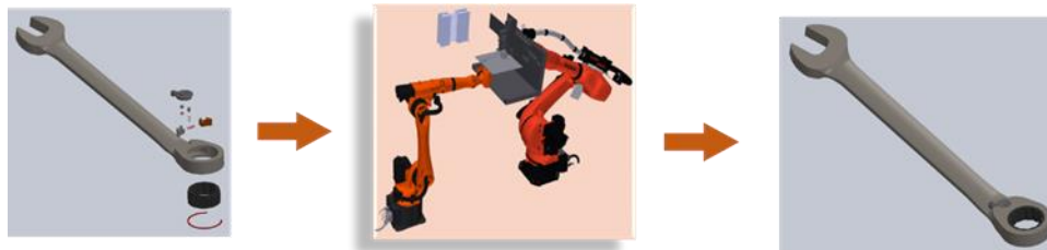
Figure 72. From the exploded-view drawing to assembly completeness via robotic assembly process
