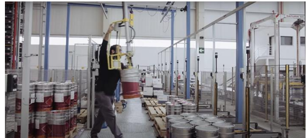
Figure 75. Operator placing a can on the pallet with the help of a material handling crane
