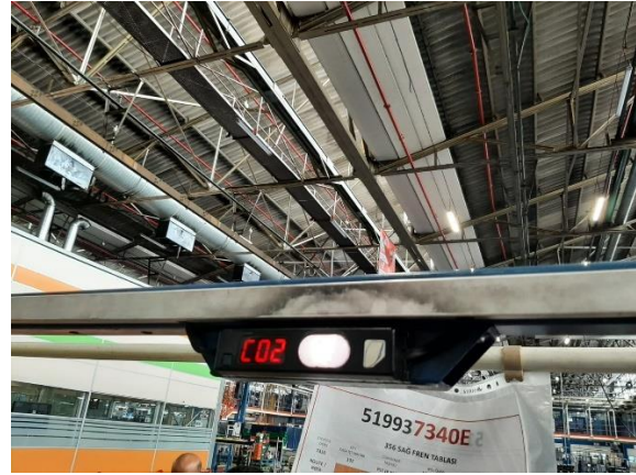
Figure 24. Pick to light device above each input container
