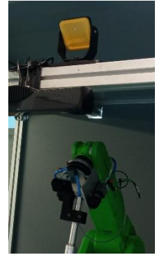
Figure 32. PSEN rd1.2 safety radar sensor
