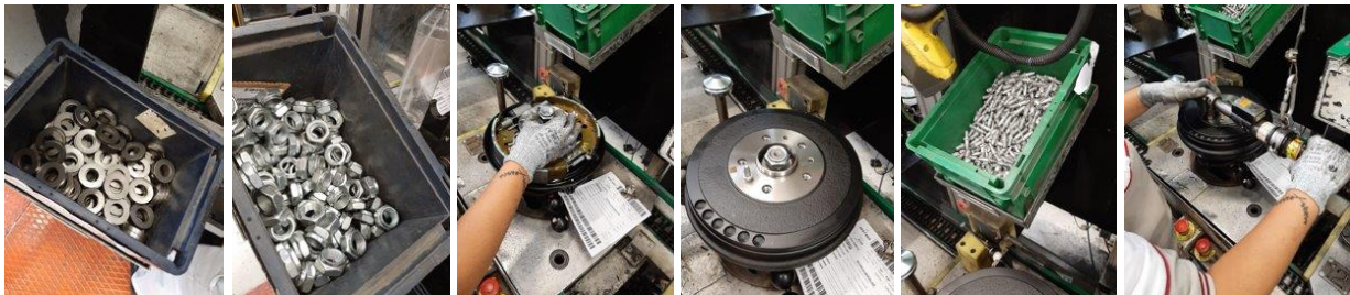
Figure 22 Use case UC2b, pre-assembly of real wheel in automotive sector
