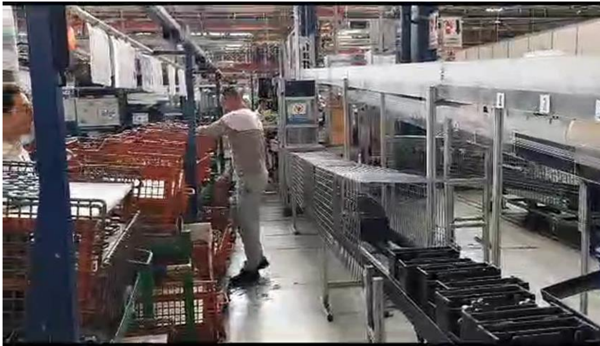
Figure 17. Operator taking a component from the input container (left side). It will then put on the destination container (right side)
