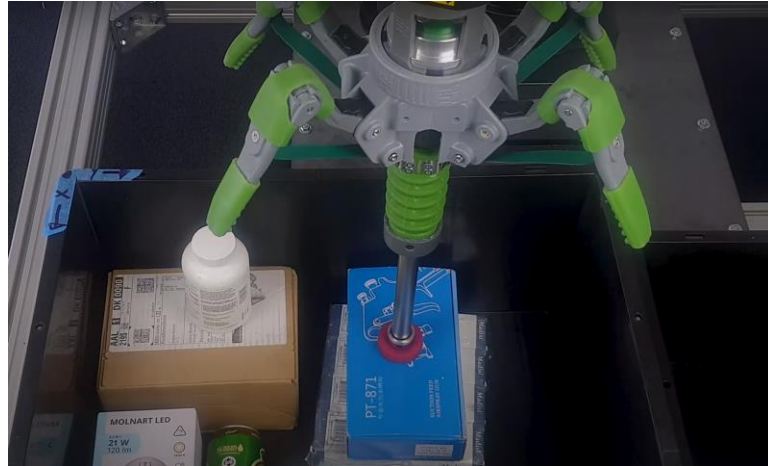
Figure 56. The combined finger + suction gripper under study
