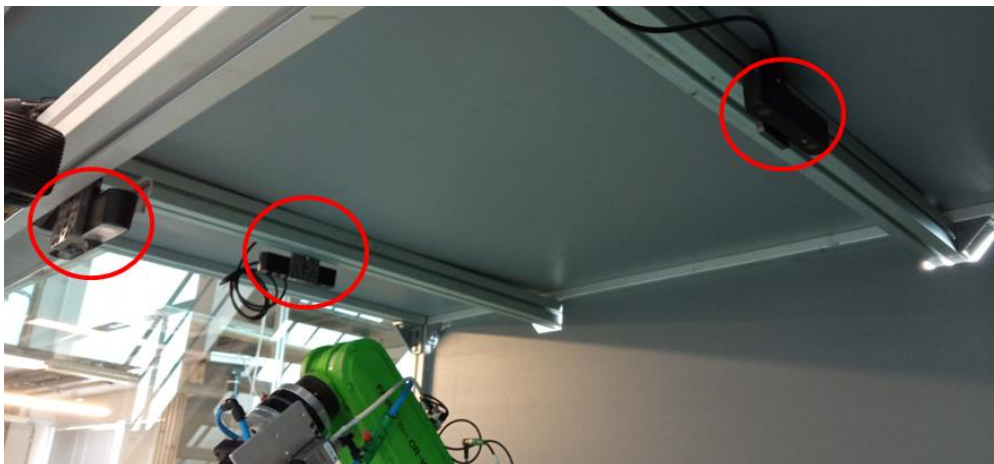
Figure 33. Detail of 3 of the ZED2i
