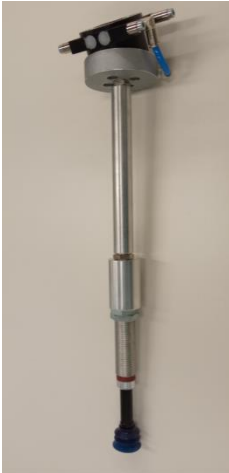
Figure 55. One of the 2 grippers with automatic quick-change mechanism
