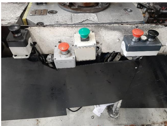
Figure 15. Push buttons to control the conveyor belt that transports the output containers
