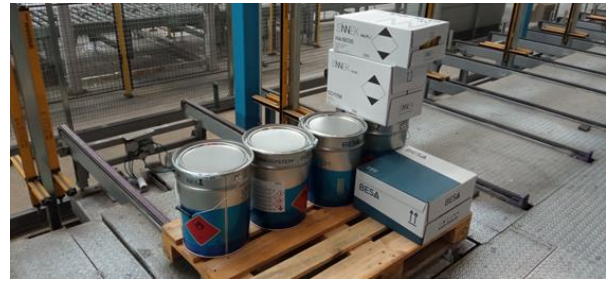
Figure 45. Example of multi-reference pallet
