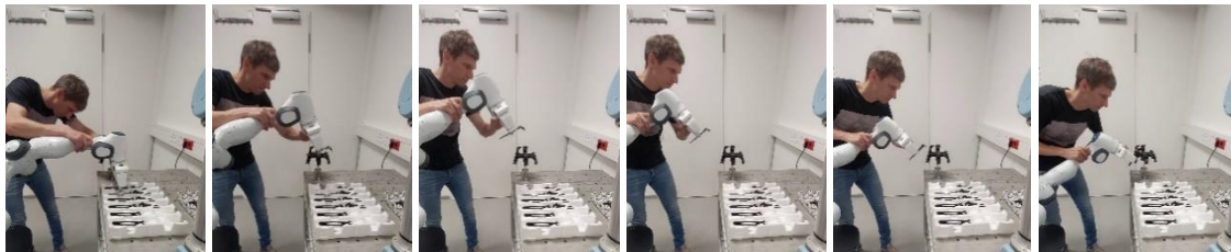
Figure 28 Kinaesthetic Teaching of an assembly task
