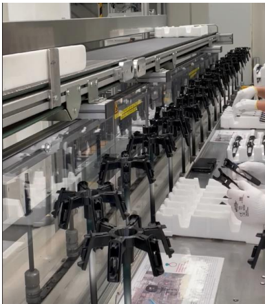
Image – fixturing at a loading/unloading station
