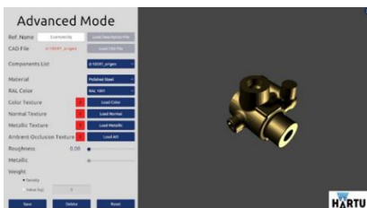
Figure 2. Interface for defining the visual appearance and physical characteristics of parts
