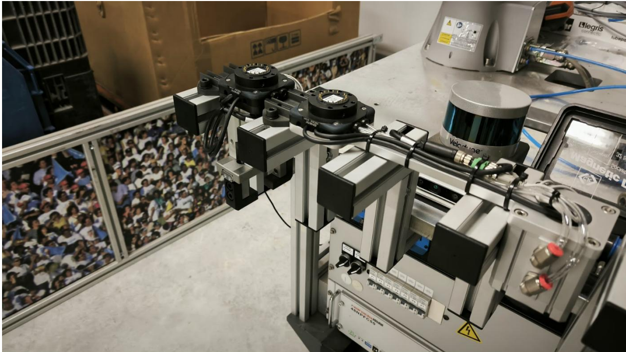
Figure 10. Tool exchange station for TOFAS UC1 and UC2a
