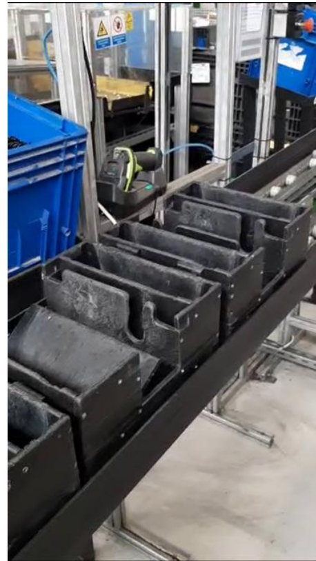
Figure 18. Destination containers on the conveyor. The blue boxes contain the discs
