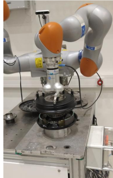
Figure 31. Dual-Arm KUKA iiwa as demonstrator for UC2b. Upper image: Dimensions; left image: actual installation; right image: gripper holding the drum brake (approx. 5.5 kg) in place for assembly on the brake unit (brake shoes, hub, spindle, back plate).
